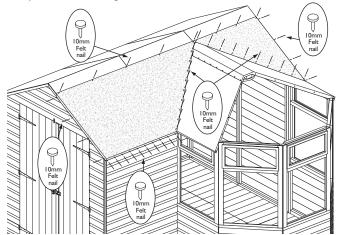
using the third 3.3m piece of felt over the ridge of the roof, ensure that it overlaps all the other felt pieces to ensure no water leaks. Secure down along each long edge using  $28 \times 10$ mm felt nails. Dress down the ends and secure at each end using  $4 \times 10$ mm felt nails a shown below.
